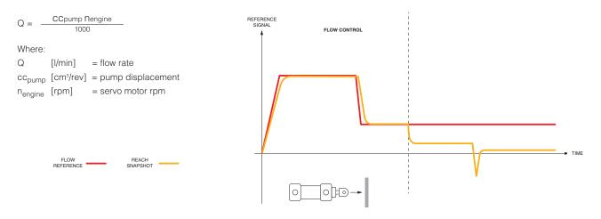
During the flow control phases the pressure reference signal is still present and has the function of limiting the maximum pressure of the system and therefore the force applied by the hydraulic actuator ensuring the safety of the machine.
