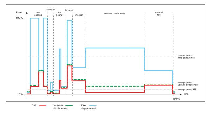
In the graph it is possible to detect in detail the great advantages of SSP in term of energy saving compared to other traditional systems. It is especially during the holding pressure phase, that you have the greatest benefits in terms of energy saving are achieved. During this phase the pump rotation speed is almost 0 as it has just to compensate for the oil leakage losses of the system (of the pump itself or of other hydraulic components), keeping the line pressure constant.
