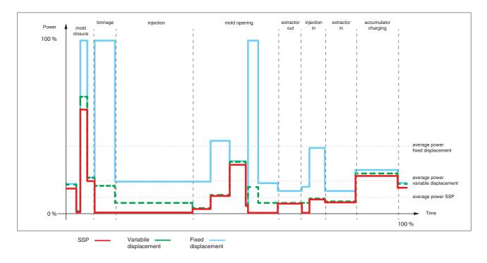
In the cycle shown in the graph, the SSP pump ensures energy savings of up to 65% compared to traditional systems.
