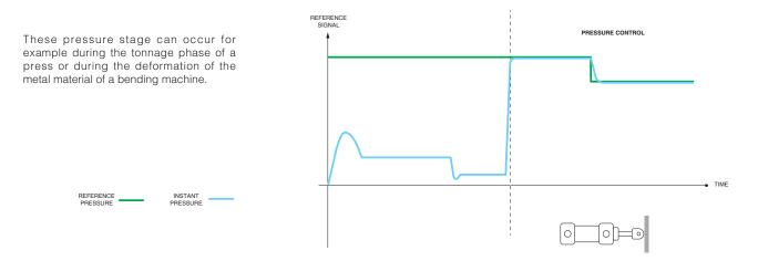
If, during the pressure control phases, a line depressurization is required, the PGI/PGIL pump is able to rotate in the opposite direction for a short period of time.
