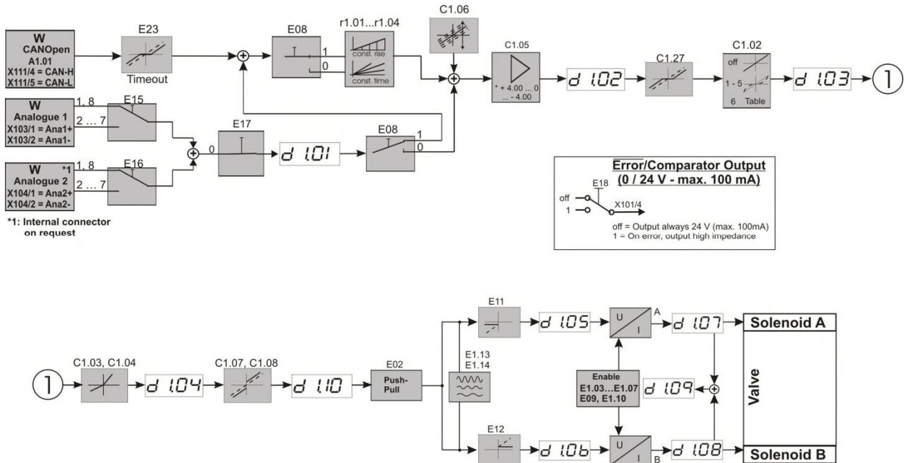
Figure 11: Block diagram mode 1
