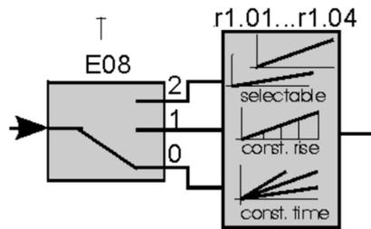
Figure 16: Object 0x6330..0x6336: Ramp function E08 r1.01..r1.04
