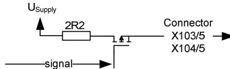
Figure 25: schematic of digital output 1
