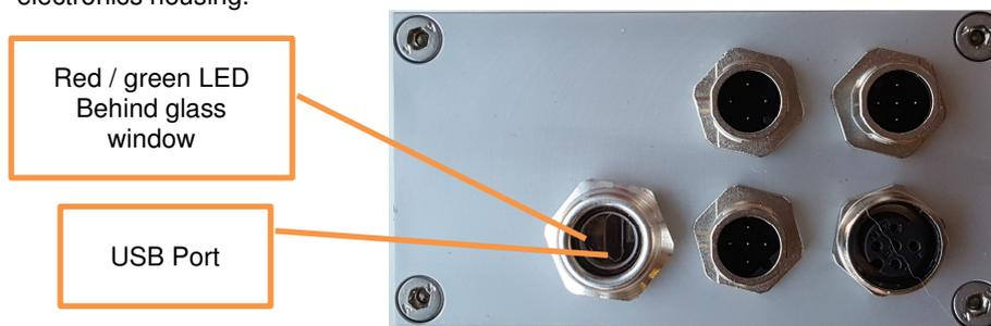
Figure 27: Top view, status LEDs and USB port
