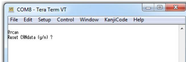
Figure 36: The reset CANopen command
