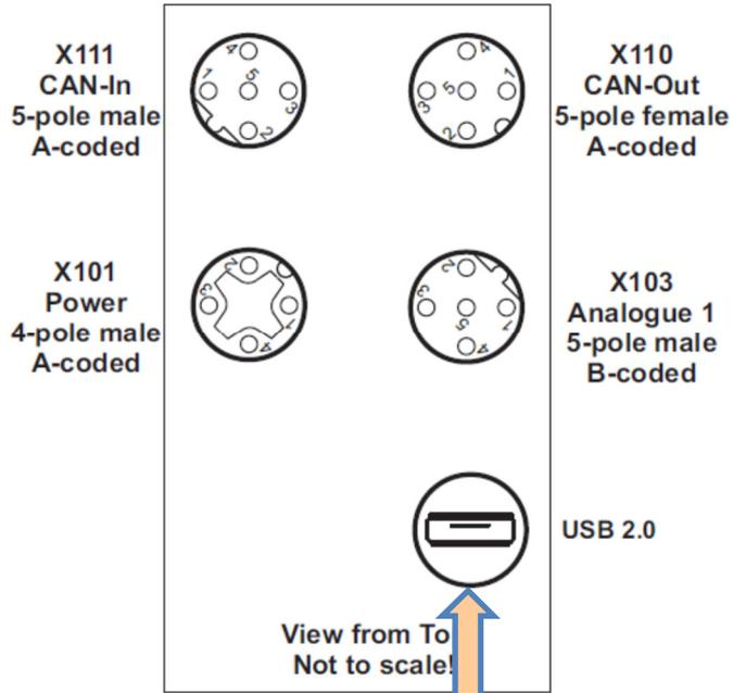
Figure 38: Connect the USB interface
