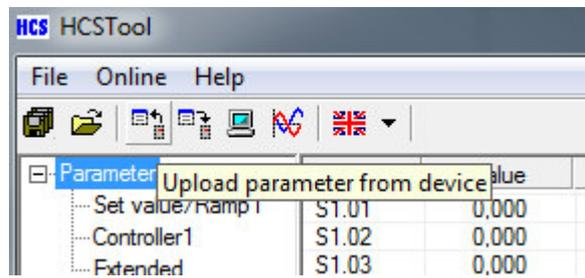
Figure 29: The upload command of the "HCSTool"
