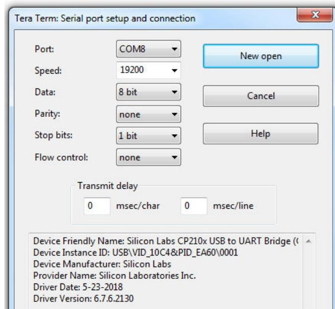
Figure 34: Setup COM port and baud rate of “Tera Term”
