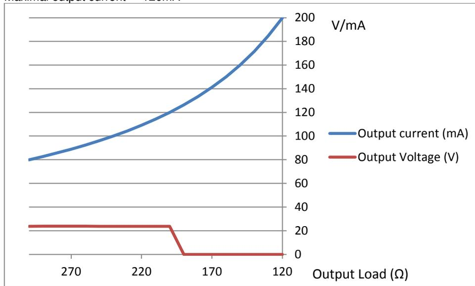
Figure 26: Diagram of output current/voltage versus resistance
