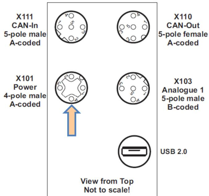
Figure 40: Connect the power to the ODC
