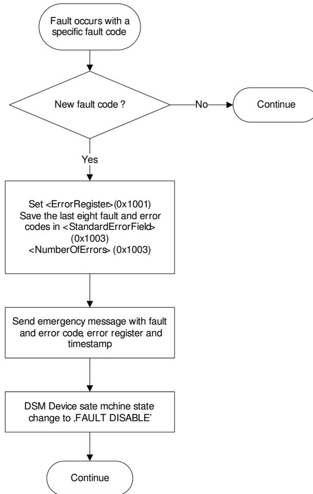
Figure 18: Fault reaction flow chart
