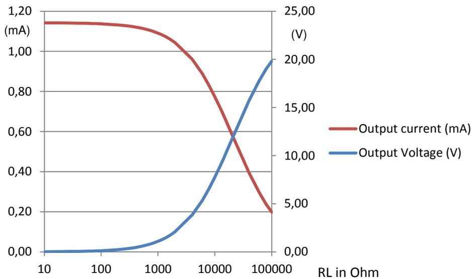
Figure 24: Output high, voltage and current curve at 24V supply
