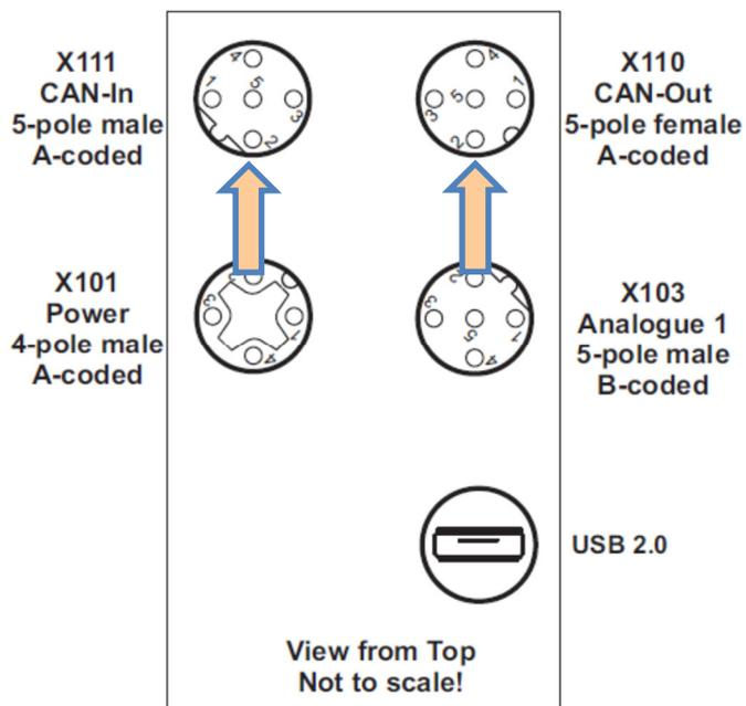
Figure 39: Connect the CAN interface
