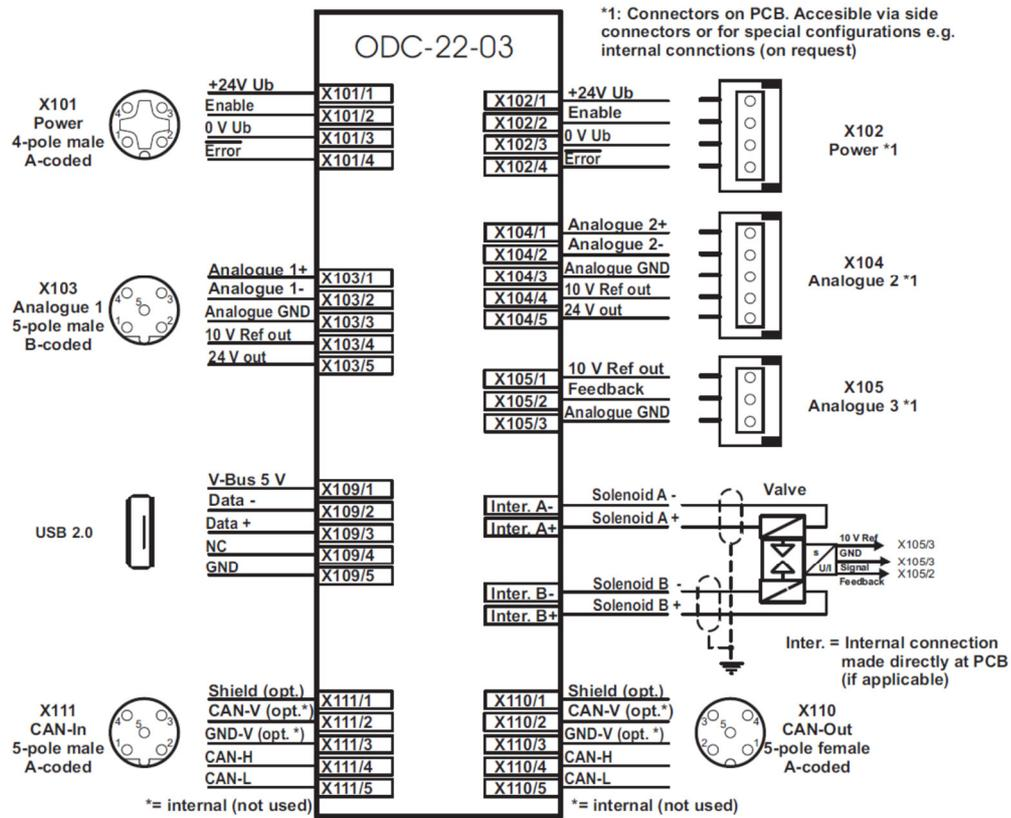
Figure 1 : Connection diagram
