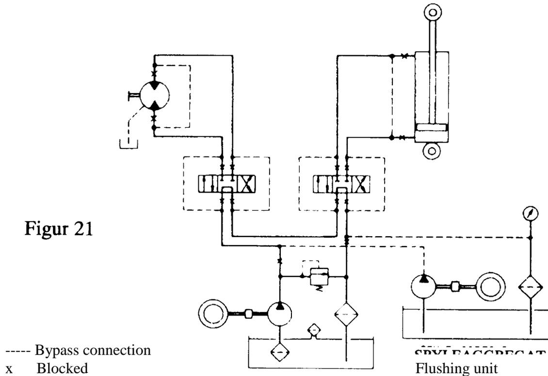
Flushing should continue as long as time allows, preferably several hours. During the process, the oil filters must be carefully monitored and filter cartridges replaced as necessary. During flushing, filters should be used which have the same filtration rating (or finer) as the filters used in the system. After flushing, all filter cartridges must be replaced. The oil is normally not changed.
