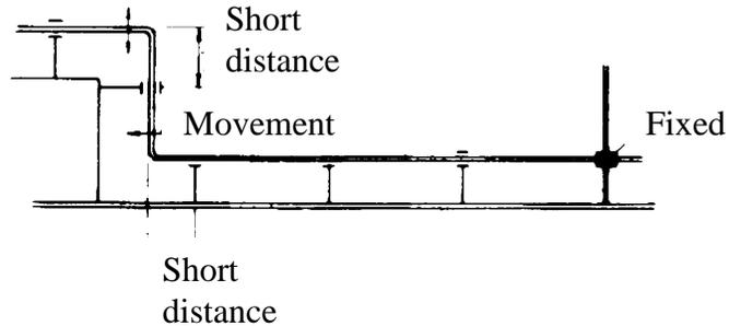
A 1 meter length of tube will expand 1 mm with a 80°C temperature increase. For long tubing distances, it is obvious that the expansion can be quite large - Table 2.
