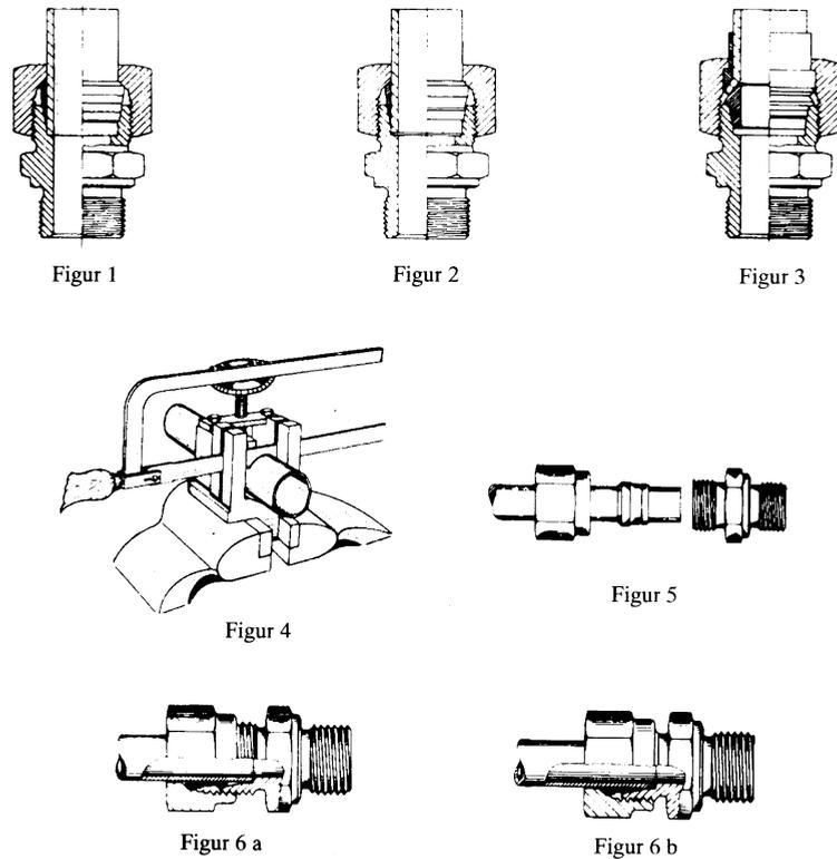
Figure 1 shows a cutting ring coupling cross section with all parts. Note the direction the cutting ring faces. The assembly procedure is as follows:
