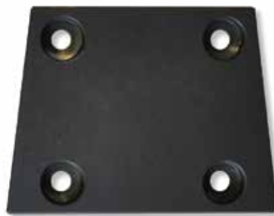
The same plate, with running-in film applied
