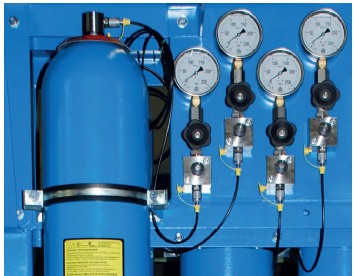
Diaphragm accumulator with mini-measuring connection
